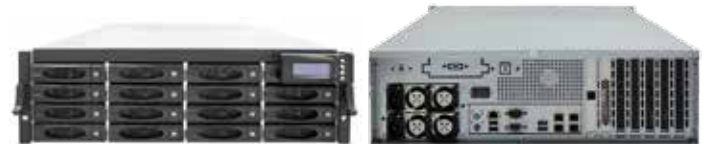
3U 16Bays Single or Dual Xeon Platform
